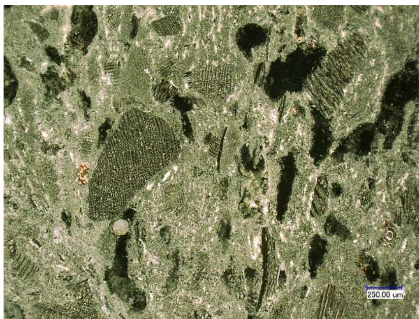
Figure 10: Optical microscopy of quartz charcoal pellets.
