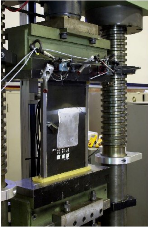
Figure 4.3.17 Failure mode of Temporary Skin Repair
