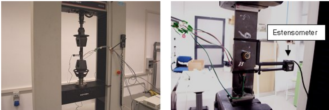
Figure 4.5.7 Extensometer used for single-lap specimens
