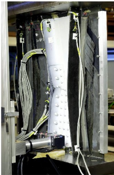
Figure 4.3.17 Failure mode of Temporary Skin Repair
