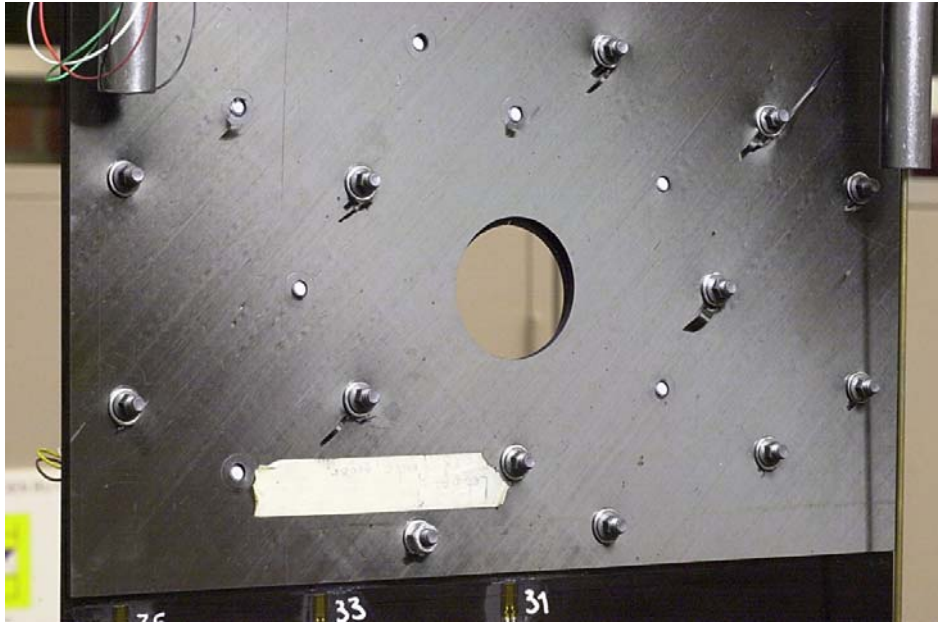
(a) Bolt Pattern 1 showing bearing failure and subsequent bolt failure
