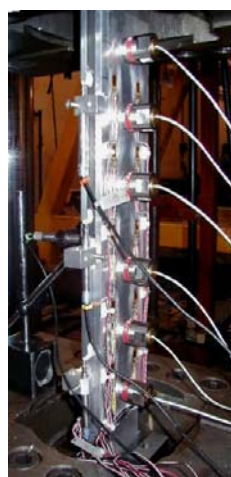
(a) Instrumented Bolts and Strain gauges
