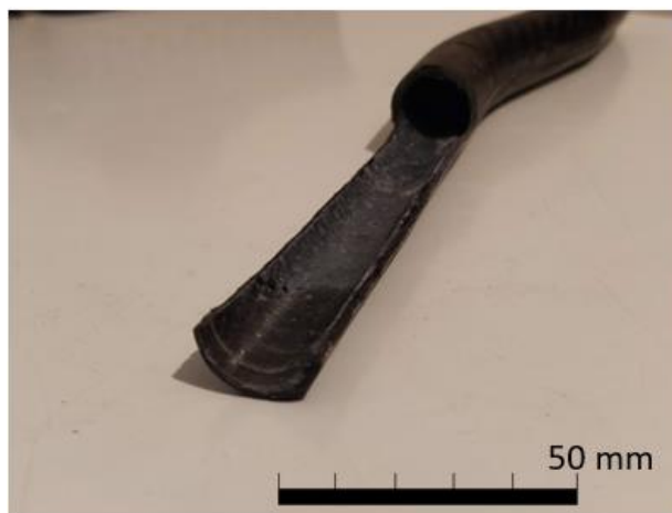
Figure 4.10 Cut away of composite shrink tape consolidated CFRP tube after the core was dissolved.
