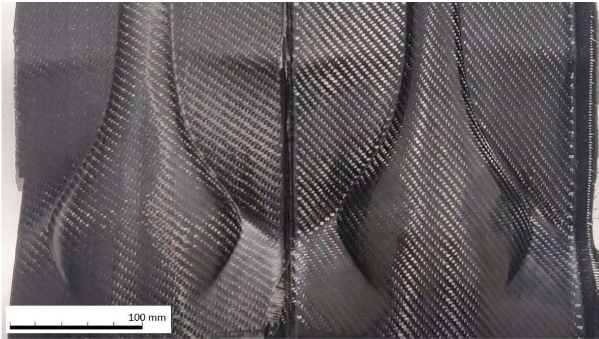
Figure A.6 A side-by-side comparison of CFRP infused parts from the matte (left) and gloss (right) thermoformed tooling.
