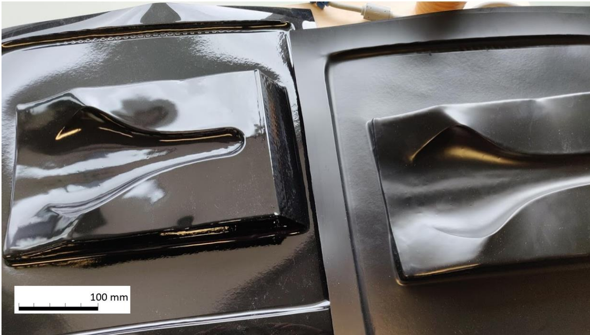
Figure A.4 Thermoformed covers of the bicycle saddle infusion tooling. Gloss (left) and matte (right).
