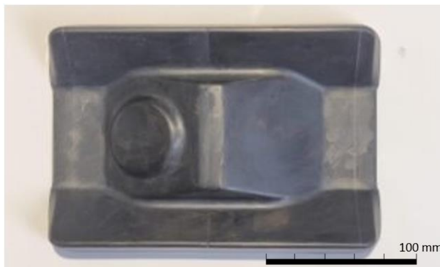
Figure 4.6 Swirling pattern from the application of Meguiar's M-08 wax on the plug tooling surface.
