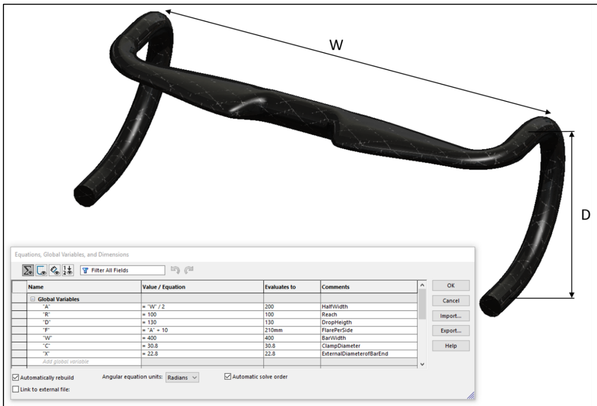
Figure C.1 Parametric driven CAD model of road bike handlebars using global variables to customise final dimensions.
