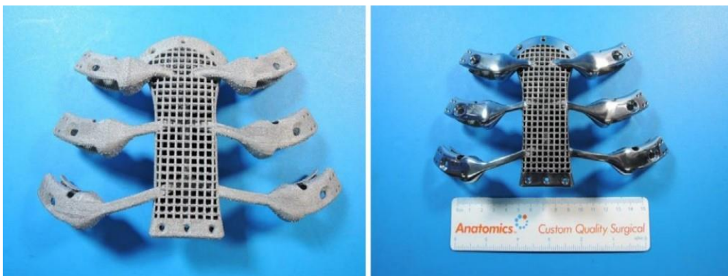
Figure 11: 3D printed titanium sternum implant post-print and post-processed (Thompson 2018; Kernavnar et al. 2021)
