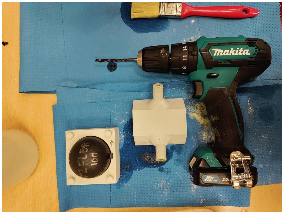
Figure 24: Drilling jig in use
