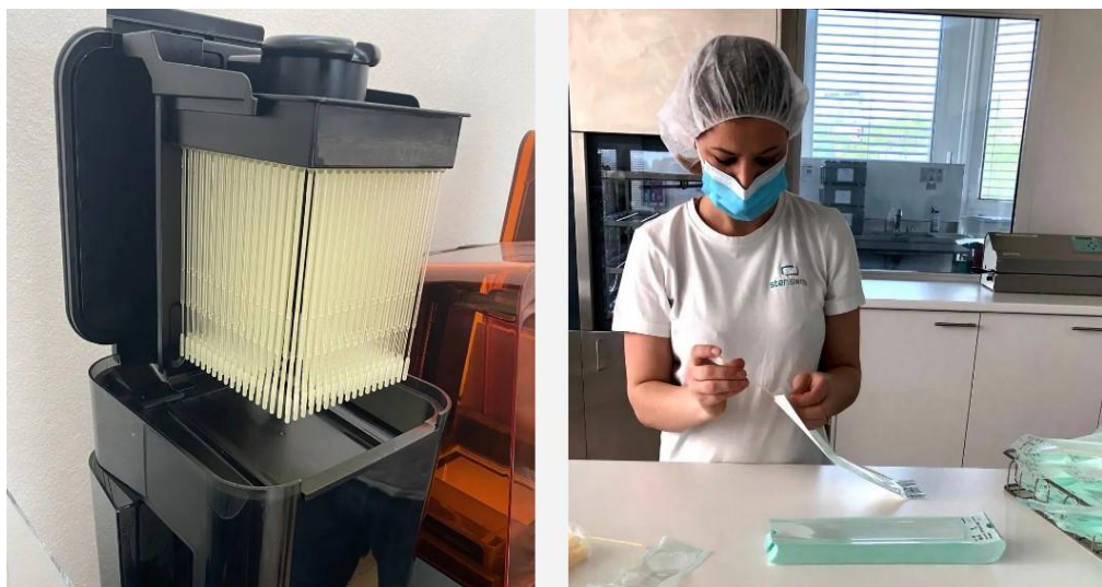
Figure 13: Formlabs SLA printed nasopharyngeal swabs post-wash and packaging (Formlabs 2020a)
