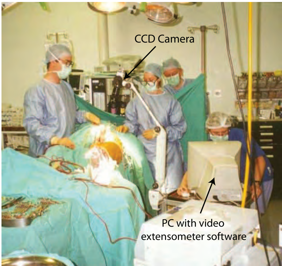
Figure 4.1: In vivo measurement set-up showing the CCD camera over the area of interest and the PC recording real time deformations.
