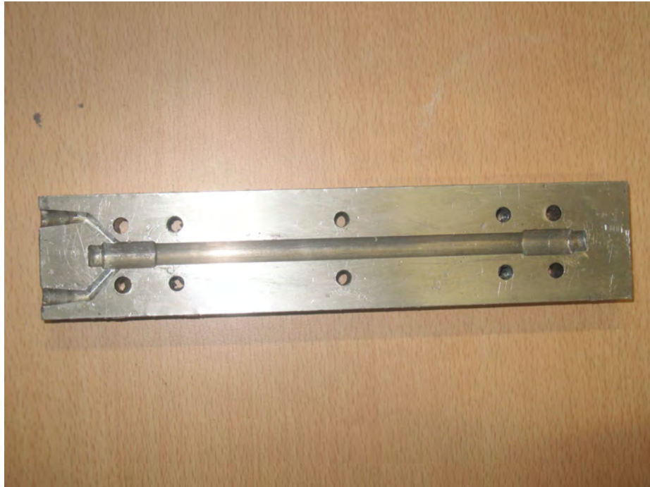
Figure B.1: Straight section mould with slots for guide pins.
