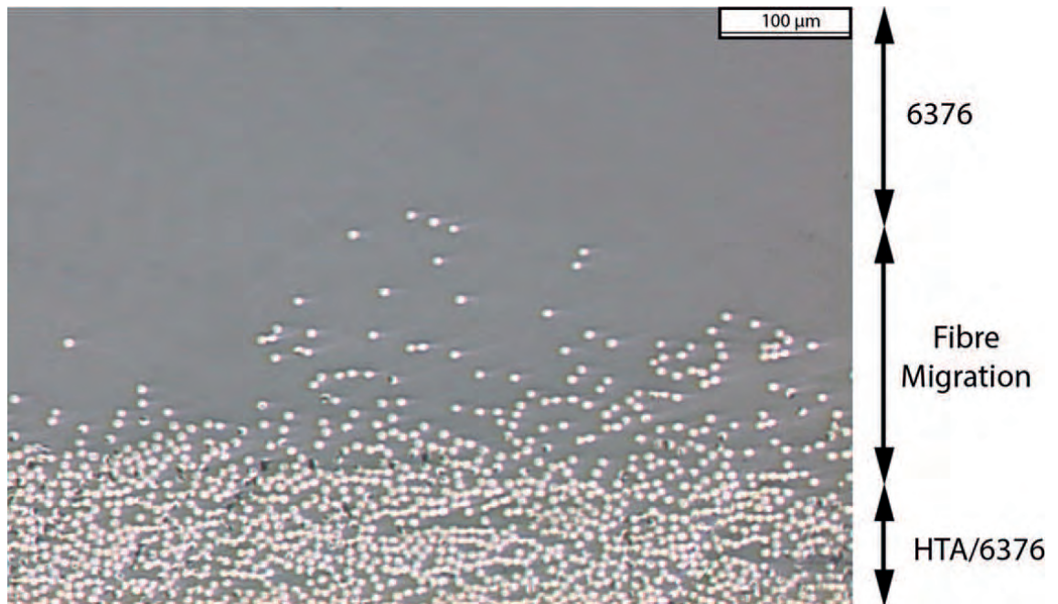
Figure 5.6: Resulting microstructure of the hybrid sample at the composite/epoxy interface
