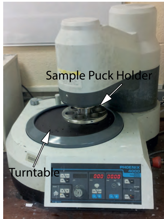
Figure 5.5: Buehler Phoenix 4000 sample preparation system
