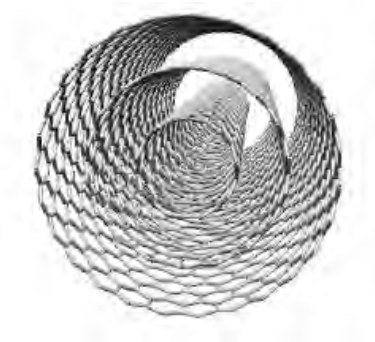
Figure 2-4: A multi-walled CNT (MWCNT) consisting of three walls.
