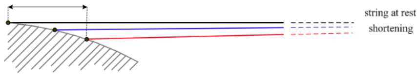
Figure 2.5: Shortening and lengthening of string due to the shape of the bridge.
