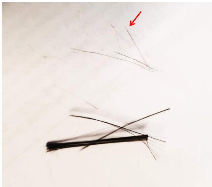
Figure 5.11 PAN based CFs breaking during separation.
