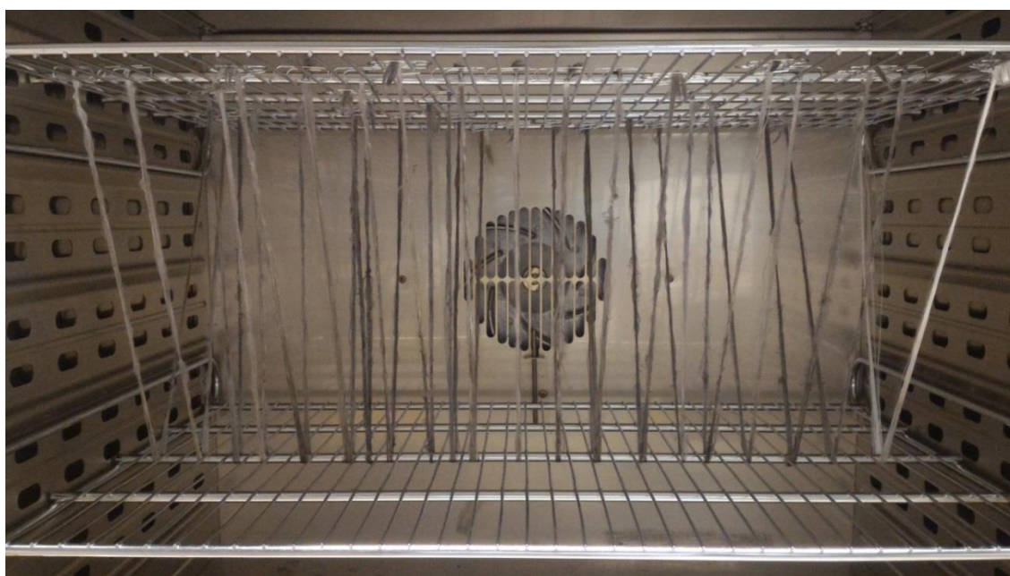
Figure 3.3 PAN precursor fibres prepared for stabilisation in a convection oven.
