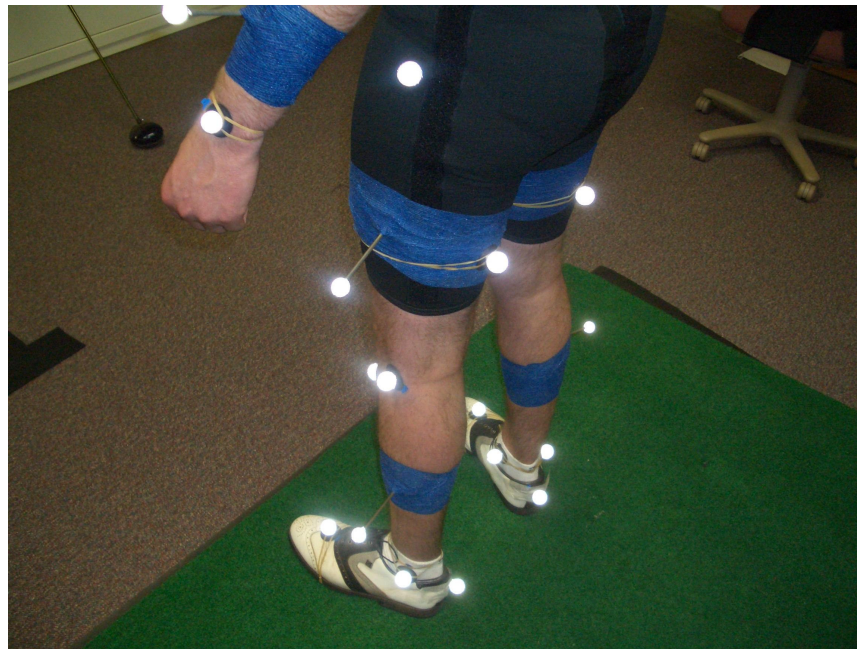
Figure 3.17 Femoral and tibial wand marker arrangement
