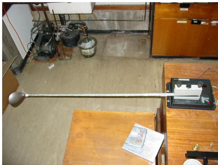
Figure 3.3 Measuring shaft frequency
