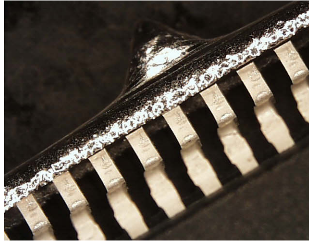
Figure 2 – QFP leads with Pb-free solder not wetting @ 221 0 C [6]
