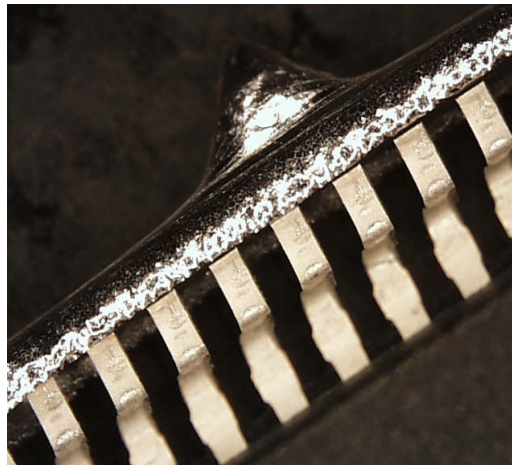
Figure 3.3 QFP leads with SN100C solder not wetting at 227°C [42]
