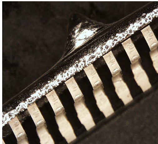
Figure 3.2 QFP leads with SAC305 solder not wetting at 221°C [42]
