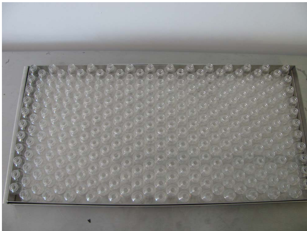
Fig. 13: Vial configuration within a given tray. The vials were placed in the form of a honeycomb structure to maximize the number of vials per tray and to maximize heat transfer by ensuring maximum vial to vial contact.
