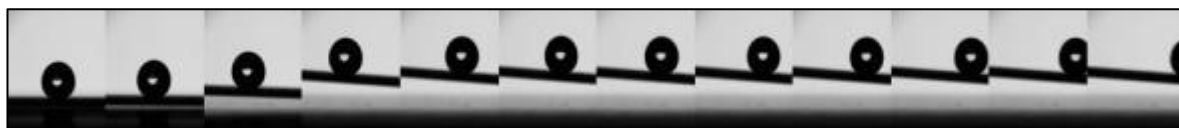
Figure 4.13 Screenshots taken during the tilting of a water form on the surface of an evaporated 20nm layer of In on carbon spheres.
