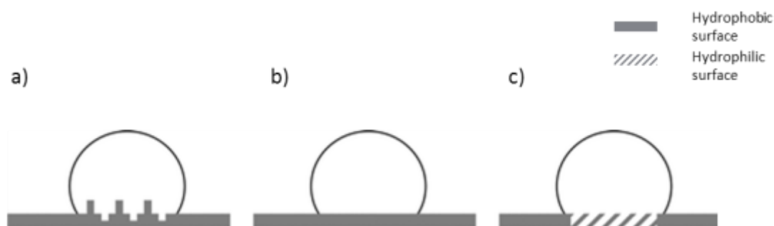
Figure 1.4 Different topography a) and surface chemistry c) (hydrophilic spot within a hydrophobic material) within a sessile drop which display the same contact angle as a smooth surface of the same material in b). 17
