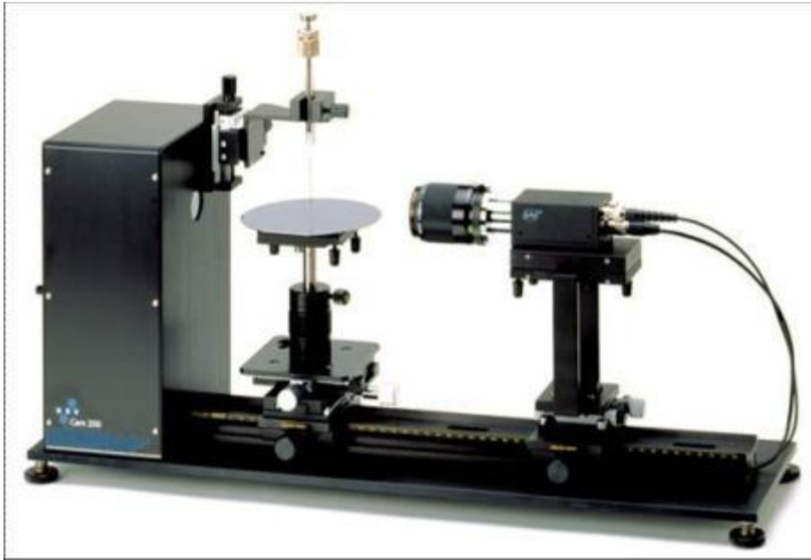
Figure 2.3 KSV Cam 300 Series with high resolution camera and adjustable stage attachments used for the measurement of contact angle and contact angle hysteresis.
