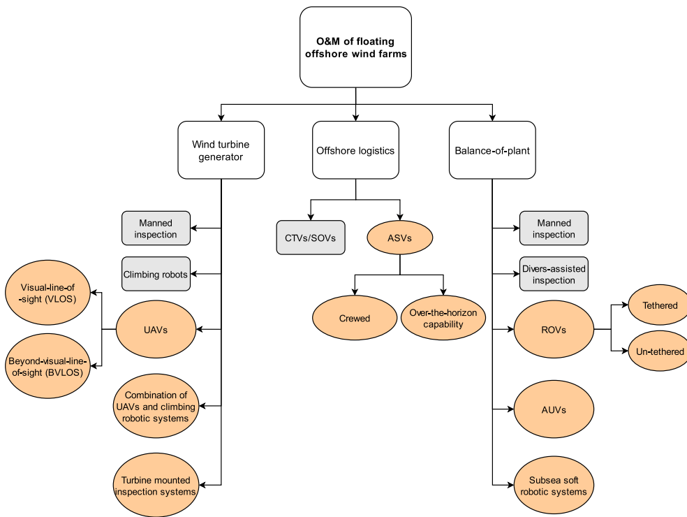
FIGURE 4 Research pertaining to robotics for O&M. rectangular areas (grayed): widely investigated. Elliptical areas (with filled color): possible research gaps
