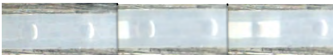
Figure 8: Still images from a video showing cross-communication due to preferential wall wetting of the solution (in this case, \text{KNO}_3 /toluene) separated by water (droplet-shaped). Time progresses left-to-right at a rate of approximately 1 second per image. Tubing inner diameter = 0.5 mm.
