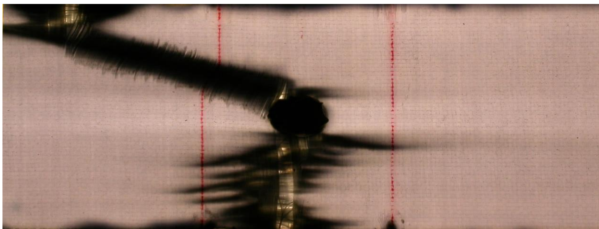
(b) Backlight visualisation of CP 3 (8 plies) open hole specimen fracture damage
