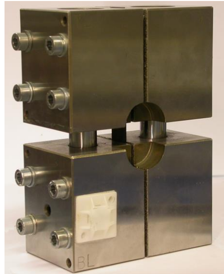
Figure 4.4 An assembled CLC rig including specimen
