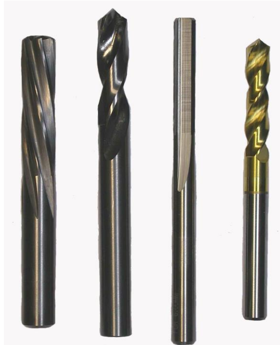
Figure 5.2 Carbide tooling for hole drilling, left to right: spiral reamer, drill, straight reamer, tin coated carbide drill
