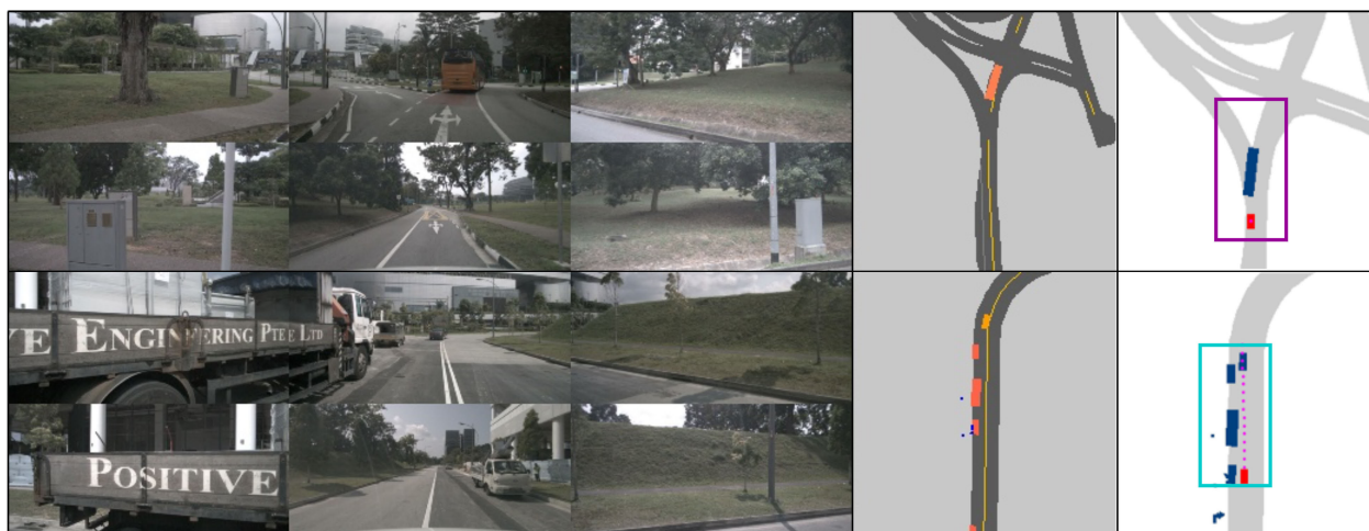
FIGURE 9. An illustration showcases a failed prediction scenario in ego vehicle trajectory forecasting using data from the NuScenes dataset. On the left side, multi-view camera images from the NuScenes dataset are presented alongside their corresponding ground truth annotations. Two failure scenarios are highlighted on the right side: the first upper scenario depicts a lack of a predicted trajectory. In contrast, the second bottom scenario illustrates a trajectory intersecting with another agent in the scene.
