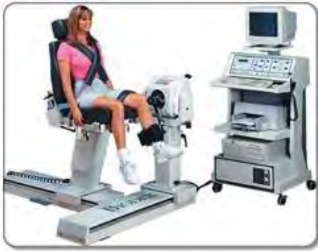
Figure 3.2: Standard isokinetic knee muscle strength testing position (Biodex Medical Systems, Shirley, NY)
