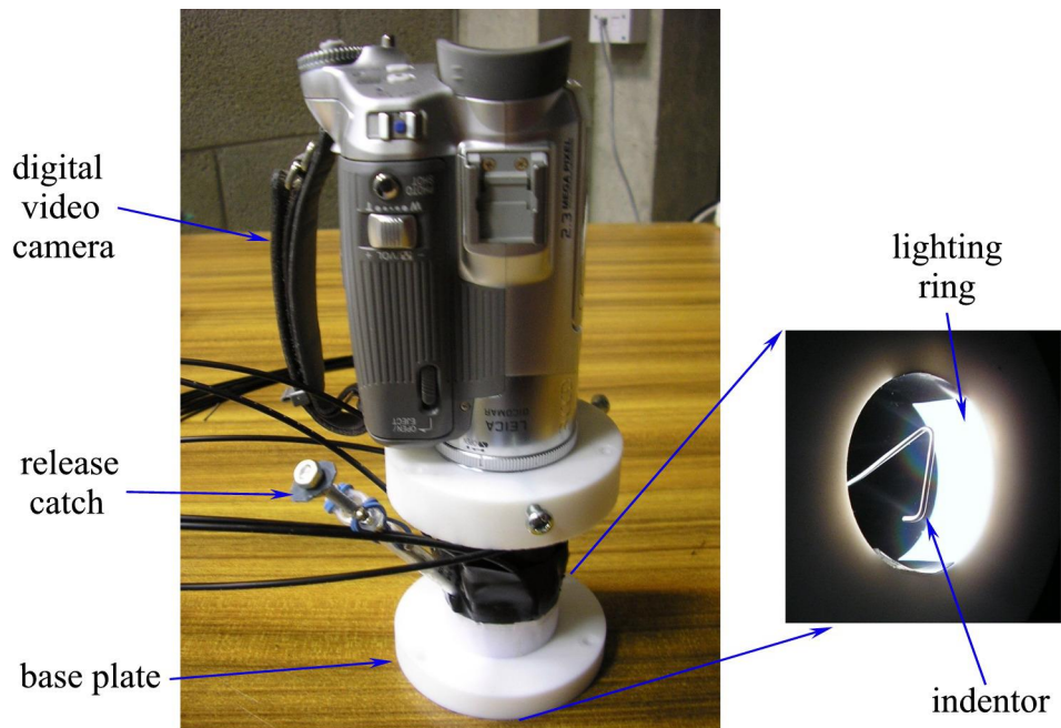
Fig. 2. Indenter and lighting system. The diffuse lighting ring and indenter are attached to the lens assembly of the camera. The base plate ensures even, low pressure contact with the skin and a flat region of interest. The indenter recoils from the field-of-view after the impression time (20 s) has elapsed.
