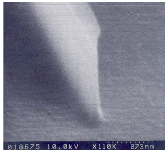
Fig. 2. SEM micrograph of 90nm isolated resist line, with 20:1 aspect ratio, formed in 1.89\mu\text{m} thick OIR-89 resist using the 2-step NERIME process.
