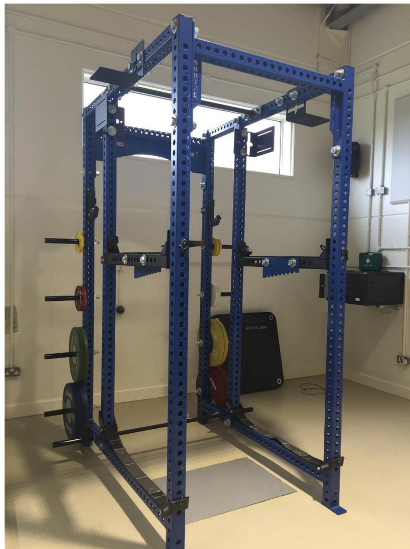
Figure 1.1 - The Sorinex (Lexington, South Carolina, USA) isometric testing rack with integrated Kistler (Winterthur, Switzerland) force plate installed in the new SII training facility
