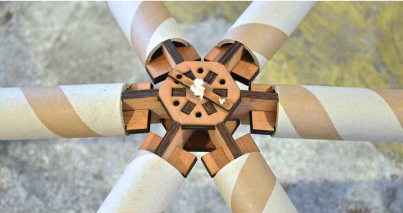
First laser cut connector prototype
