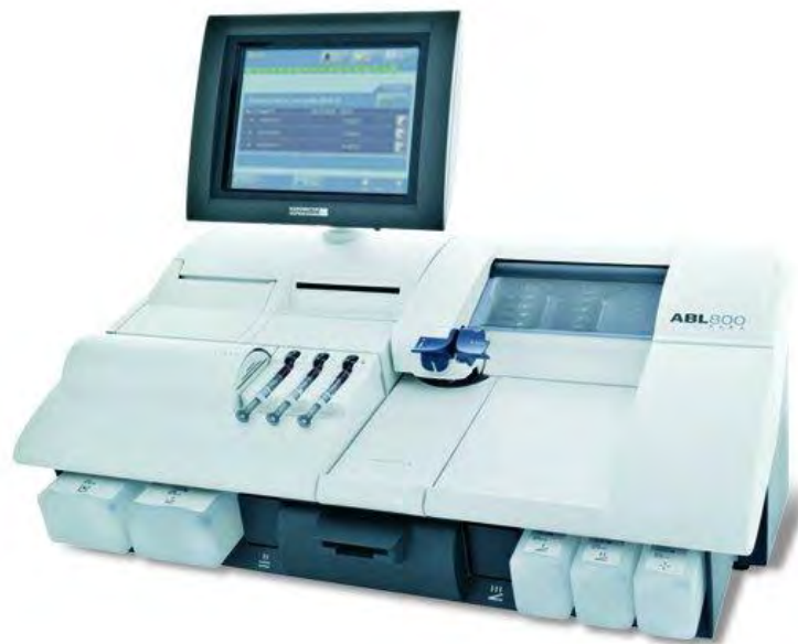
Figure 2-1: ABL800 Flex Blood Gas Analyser from the company Radiometer [96]
