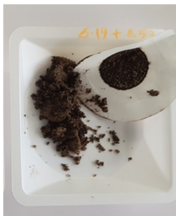
Figure 4. PA batch crystallized in the presence of the PAP impurity.
