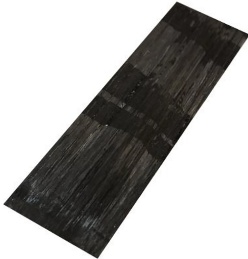
Fig. 4. Colour differences between stable and unstable crack growth (Note: the specimen is 25 mm wide).
