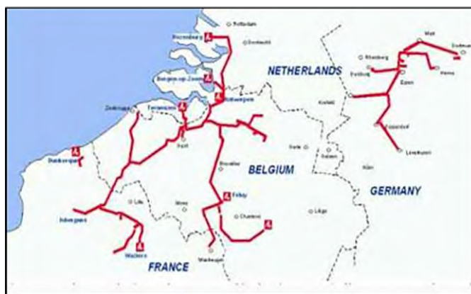
Figure 2.1 Hydrogen pipeline infrastructure currently installed in Europe. A decentralised hydrogen energy system is considered for Ireland due to lack of existing infrastructure [24].
