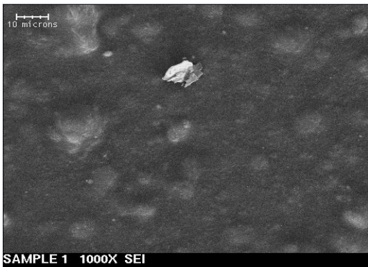
Fig. 3. SEM micrograph of thick film EC sensing layer – Magnification 1000x.
