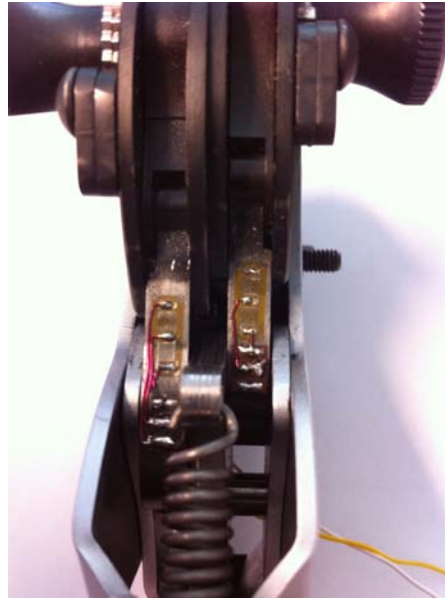
Figure 7.3: Coupling bars with strain gauge application
