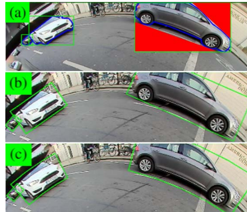
Fig. 3. Standard bounding box is not a good object representation for fisheye images. (a) Red pixels within the bounding box show a large area that does not contain the object. Oriented box (b) and curved bounding box (c) are better representations [14].
