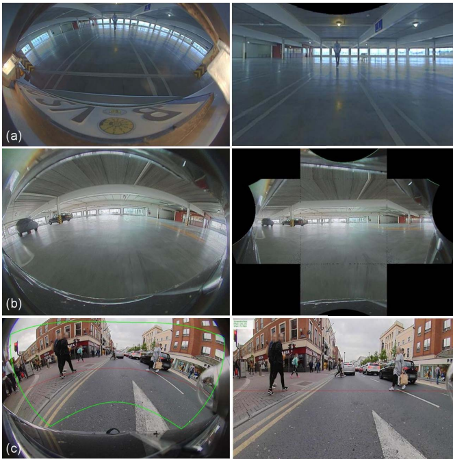
Fig. 13. Undistortion of fisheye images: (a) Rectilinear correction; (b) Piecewise linear correction; (c) Cylindrical correction. Left: raw image; Right: undistorted image.
