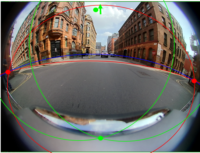
Fig. 11. Illustration of horizon line, vanishing points, and epipolar lines. Lines in the fisheye image can be approximated as conics. Equivalent to how parallel straight lines in a perspective image converge at a single vanishing point, parallel straight lines in a fisheye image converge at two vanishing points. The two vanishing points, when raised to the unit sphere, are antipodal points on the sphere. Red and green denote the perspective of horizontal parallel lines (with blue as the associated horizon line) and vertical parallel lines respectively. The red and green dots denote the vanishing points with one of the vanishing points outside the image.
