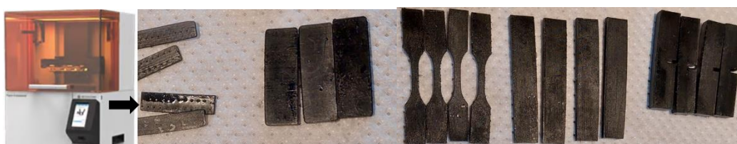
Figure 2. Figure 4® printer and 3DPd specimens.
