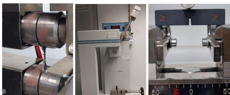
Figure 3. Specimens under tensile, Impact and SENB tests
