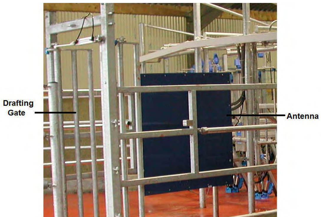
Figure 4.2: Dairymaster ® Auto-ID Antenna Mounted on Drafting Gate
