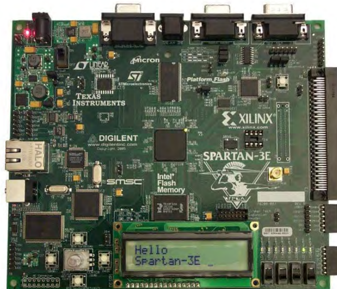
Figure 7.2: Xilinx ® Spartan 3e Starter Kit [2]
