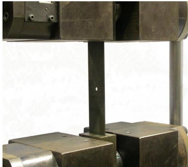
Figure 2 Open hole tension specimen clamped in the straining frame grips
