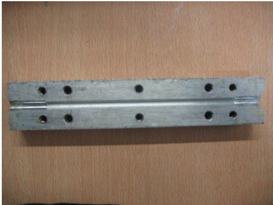
Figure B.2: Straight Section Mould for wax core
