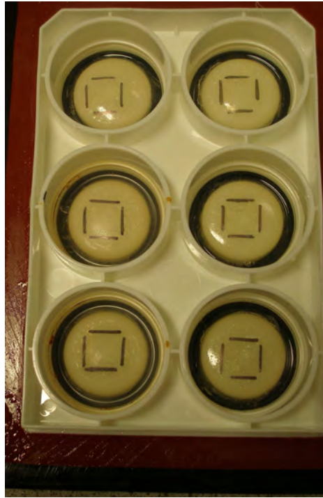
Figure 5.3: 6-well Bioflex® plates marked for calibration of the Flexercell® system.
