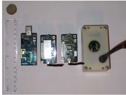
(b) Example pictures of sensor nodes, from left to right: a Tmote Sky (Moteiv Corporation, 2006), a Iris (MEMSIC Inc., 2010a), a MICAz (MEMSIC Inc., 2011), and a MICA2 sensor node in its housing (crossbow technology, inc, 2003).
