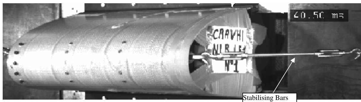
Fig. 3.1 Stabilising Bars used in NLR LE structure tests
